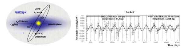
Fit count rate with  $S_0 + A \cos \omega (t - t_0)$
