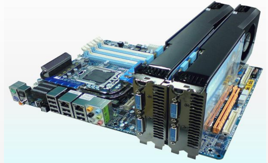
Two Nvidia GPU cards in one motherboard
