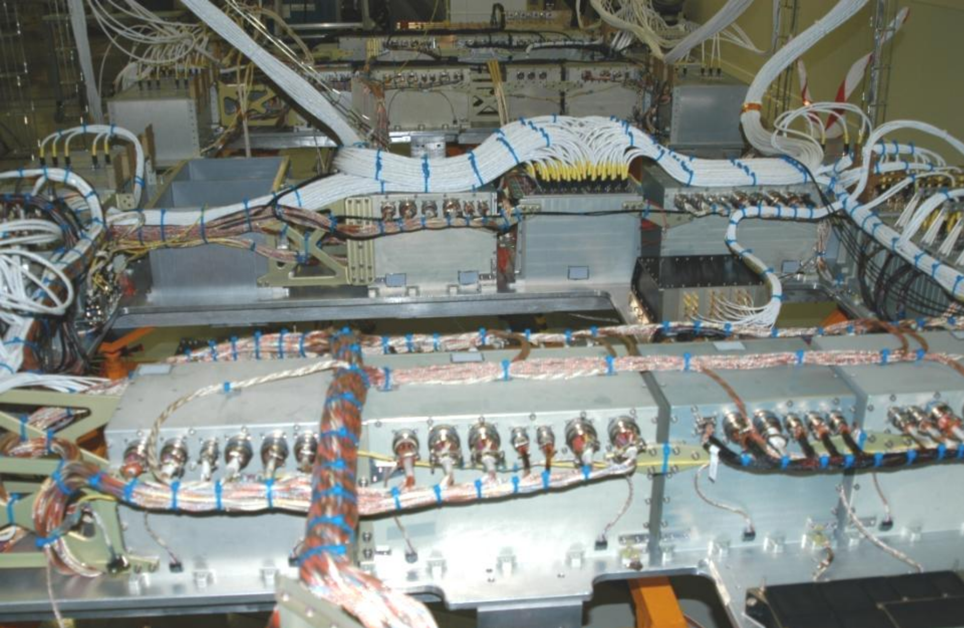
The completed flight electronics (650 microprocessors, 300,000 channels)
